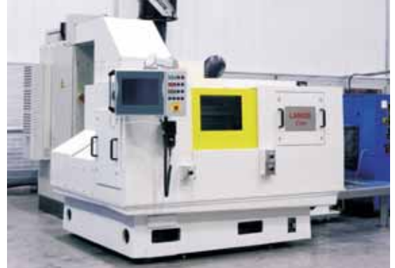
CNC6400 on Landis Lt1 Cam Grinder
