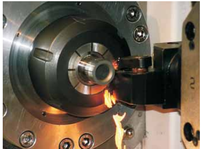
Hard Turning on the DeltaTurn 40
