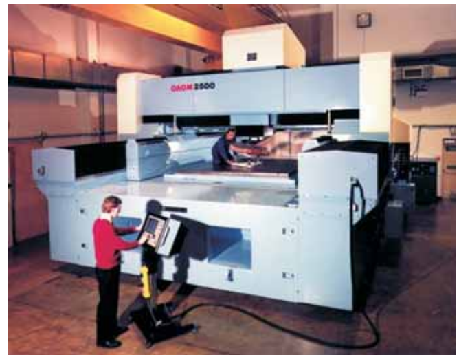
26 Tonne Bridge Driven by Friction Drives
