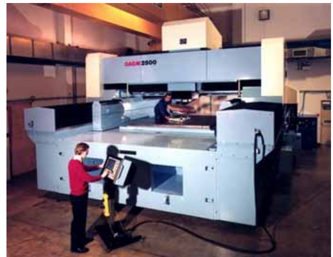
26 Tonne Bridge Driven by Friction Drives
