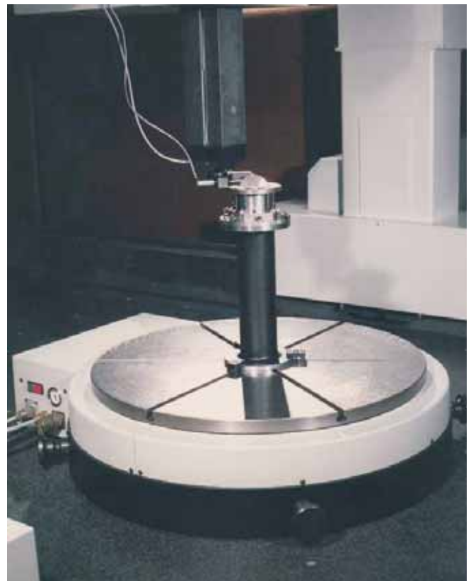
Measuring Tilt Error
