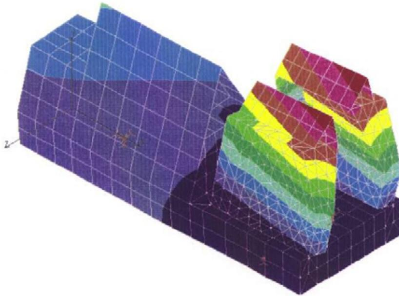
This is the first frequency which has relative motion between the grinding and wafer mount spindles. The wafer mount spindle is stationary during this vibration mode, the grinding spindles are vibrating in the direction of the arrow.
