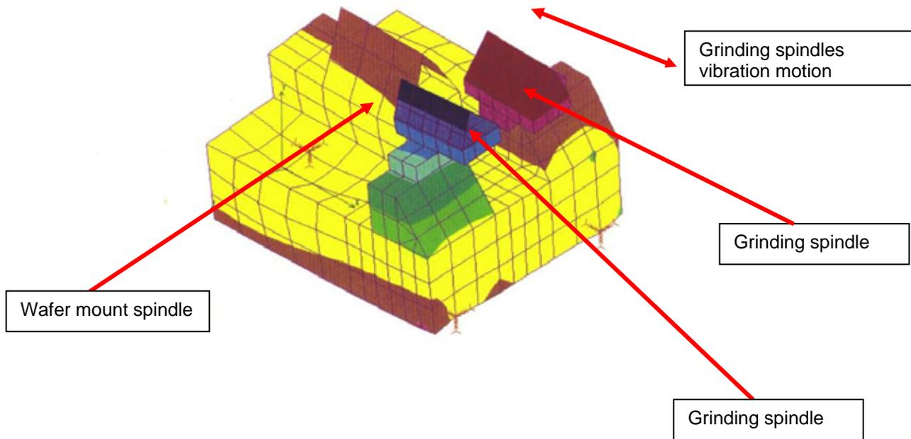
This is a finite element plot of a conventional machine.
