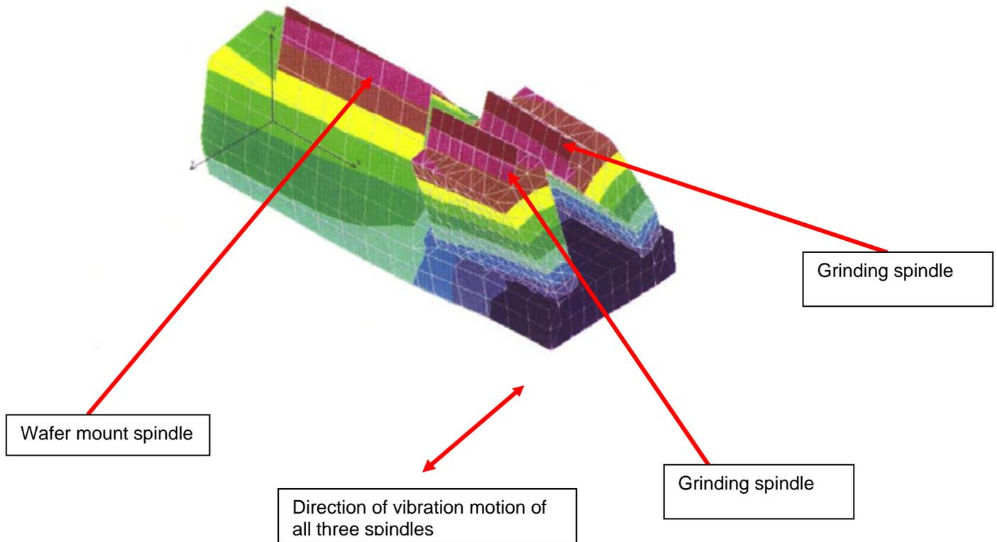
This is the first natural frequency of the SiWEG machine. The model predicted that this would occur at 85Hz. Note that the three spindles are all red indicating that there is little or no relative motion between them. Thus there is little or no damage induced in the wafer when the machine vibrates at this natural frequency.
